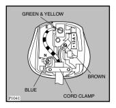
The wire coloured green and vellow must be connected to the terminal marked with the letter «E» or by the earth symbol  $\frac{1}{2}$  or coloured green and yellow.
